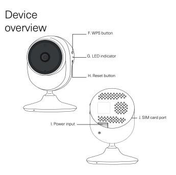
Insert the power cable (B) into the power input (I) on the camera. Then insert the power cable (B) into the power adapter (C). Plug in the power adapter (C) to a wall socket.
