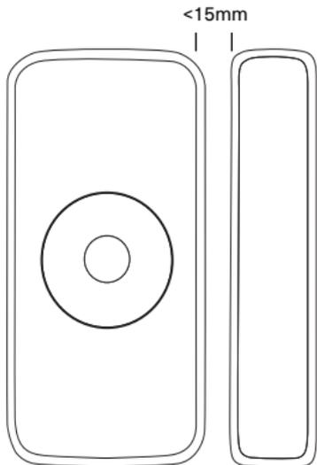
Remove the protective layer on the double-sided tape on the **device (A)**. Place the device on the wall or door/window frame.
