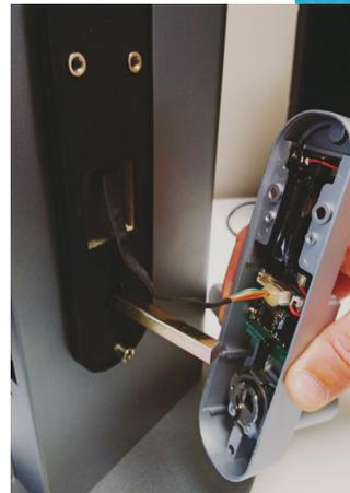
On locks with Euro cylinder, fasten the mounting bracket by using 3 of the supplied machine screws from the back. The top 2 screws should be the same length as the door thickness. The lower one should be 2 threaded pieces longer than the thickness of the door.
