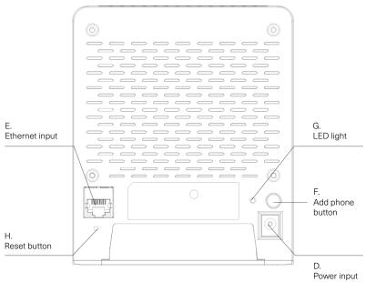
1. Connect the Ethernet Cable (B) from the Hub (E) to an internet-connected home router's LAN port
