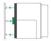
10. Find the small marking at the edge of the backplate and align it with the hole in the cover ring surrounding the door lock, Now you are sure to hit the notches on the backplate with the door lock.
