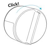
12. Activate the batteries. Pull out the plastic tab to activate the batteries. A light will flash to confirm the door lock is ready. Note: If the batteries are disconnected, you will have to re-calibrate the door lock.
