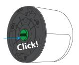
Fit the door lock over the backplate with the battery cover facing down, the tailpiece sliding into the adapter and the backplate notches into the back of the lock.
