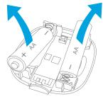
**2.** Replace the batteries respecting the polarities.
